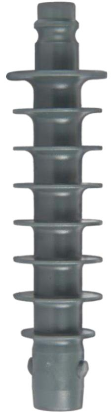
The **D18C** is designed with a quick connector for use with low pressure pumps. By omitting a valve **the outlet at 8mm is downright huge** and suitable for use with large quantities or mineral grout with coarse grit, making the **D18C** your **first choice** for filling cavities in the ground or behind walls in basements or tunnels. The huge outlet allows free flow which avoids a segregation of the material.
