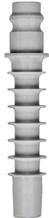
The **D12C** is designed with a quick-coupling for use with low pressure pumps. It is also suitable for use with straight mixer tips (e.g. Sulzer® Mixpac™). The **valve passage is larger, at 2.4 mm** (by about 50%) than that of any other commercially available packer.
