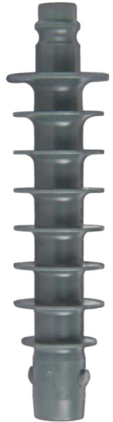
The **D18CF** is designed with a quick connector for use with low pressure pumps. The spring-loaded valve with a **passband of 4.5 mm** is suitable for filling large volumes with viscous materials or mineral grout, making the **D18CF** very versatile.
