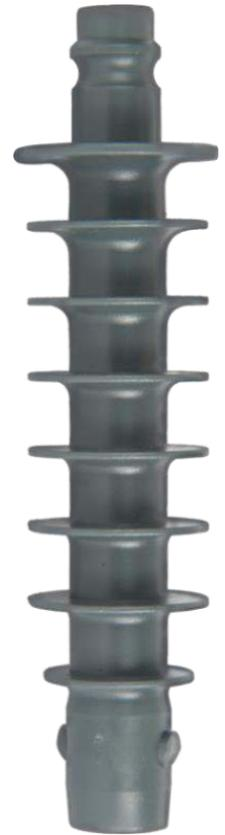
The **D18CX** is designed with a quick-coupling for use with low pressure pumps. It is also suitable for use with straight mixer tips (e.g. Sulzer® Mixpac™). The passage of 5 mm is suitable to e.g with a spear (∅ 5mm) **perform multistage injections**.
